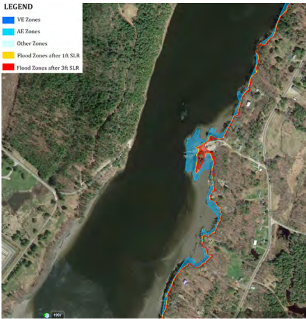
Figure 14.12 Impacts from a 100-year Flood and Sea Level Rise Wright Landing
