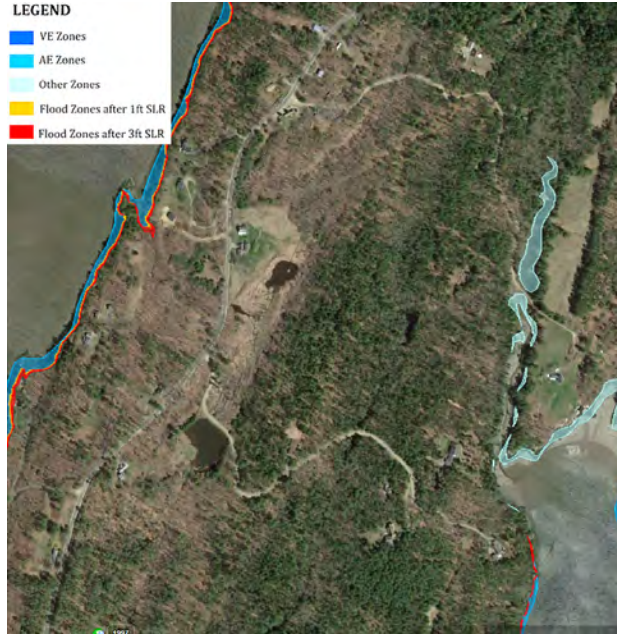
Figure 14.11 Impacts from a 100-year Flood and Sea Level Rise Baker's Road at Mill Pond
